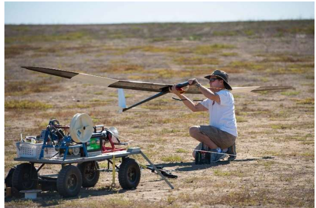
Mark Canfield demonstrating winch launch technique
