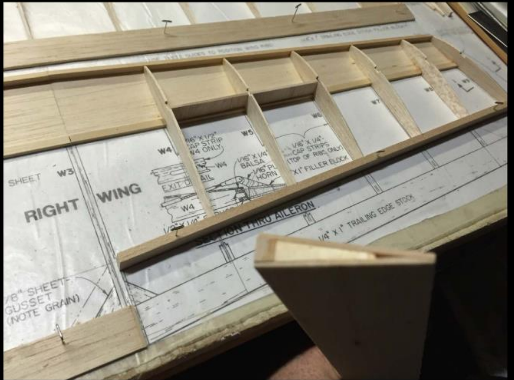
Another view of the aileron cross section showing the construction method employed.
