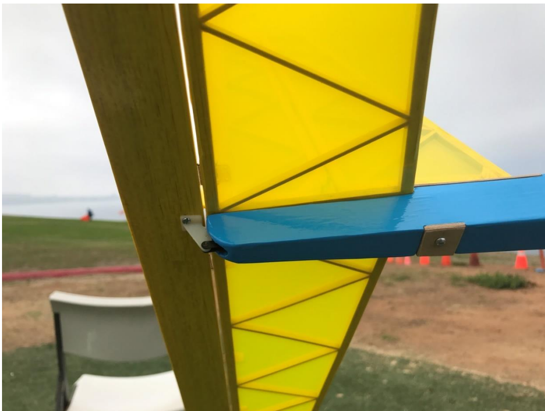
Detail at the underside of the tail showing the through-bolt connection for the fin
