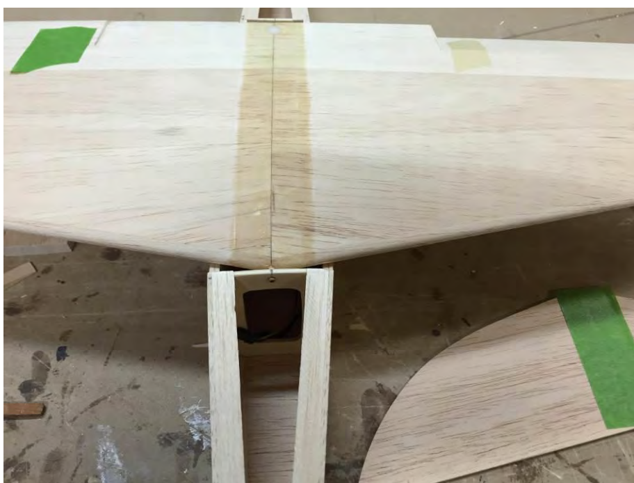
Drill out for wing hold down dowel at L.E. Fiberglass reinforce wing joint. Then glue in dowel.
