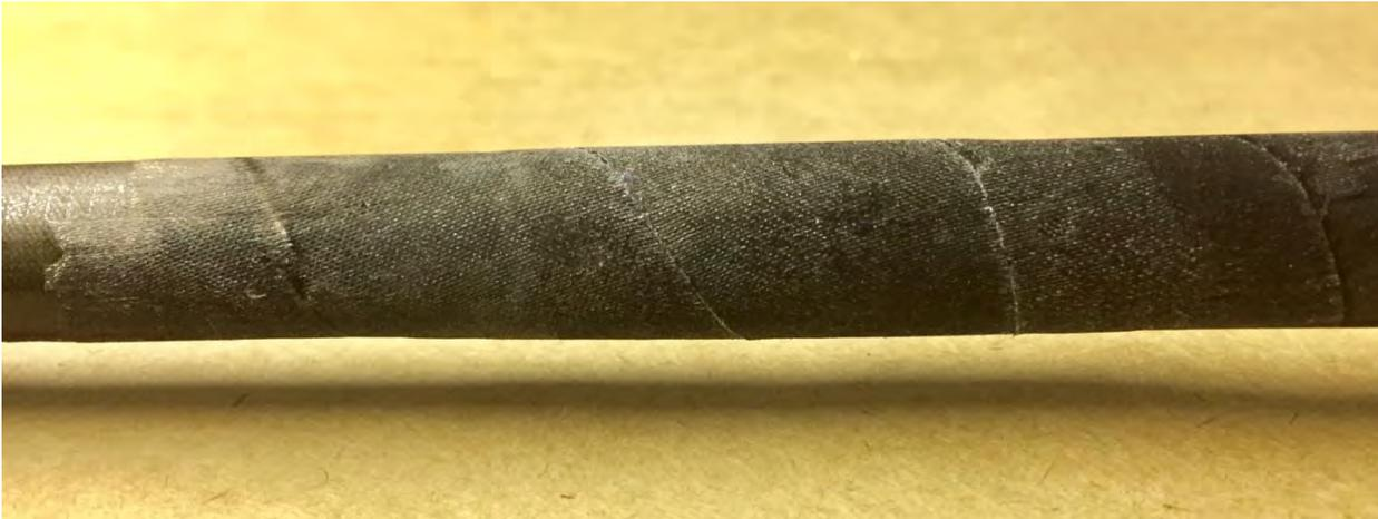
The joint turned out great! The tows were nicely compacted and merged, leaving a nice, neat, strong joint. I lightly sanded the joint to remove the fabric pattern and then finished it up a bit with some 1200 grit sandpaper. Bend testing showed that it was plenty strong; a successful repair.
