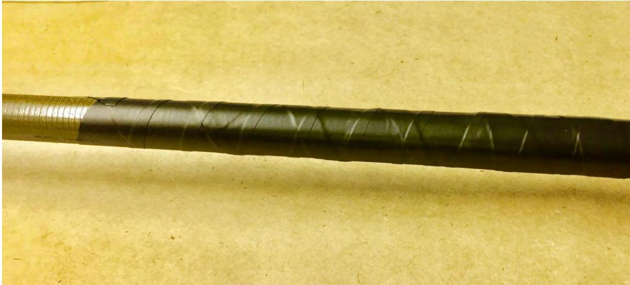
After the epoxy was fully cured (check the mixing cup - you want it completely cured and glassy), I unwrapped the electrical tape and pulled off the peel ply. Notice how much epoxy has been absorbed by the peel ply - this is dead weight that is no longer in the joint.
