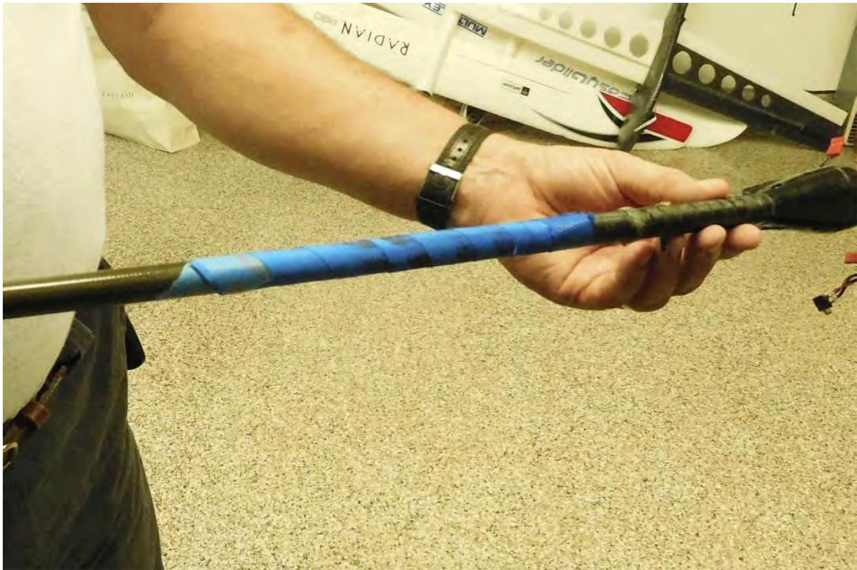
After the Peel Ply layer, we used electrical tape to compress everything tightly against the boom, winding it in a spiral pattern until the entire joint is covered. It's important to compress the joint to get the best possible bond. At this point we're done until the epoxy cures; 6 to 10 hours, depending on which hardener you use and the temperature.
