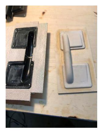
Side by side photo. The cast can be cleaned up a bit if needed. For mine, it was smoothing out the area where there was a chip in the original cover.
