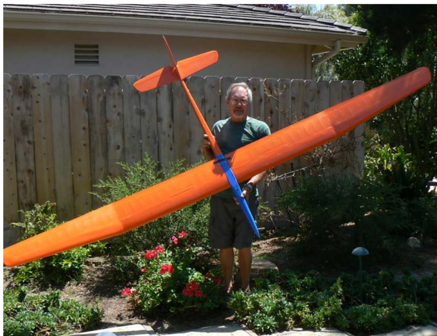
Above: This is Oly!!! before her maiden voyage launch at the Poway T/D field. Wingspan is 132", length 64" and weight 3# 14 oz.
