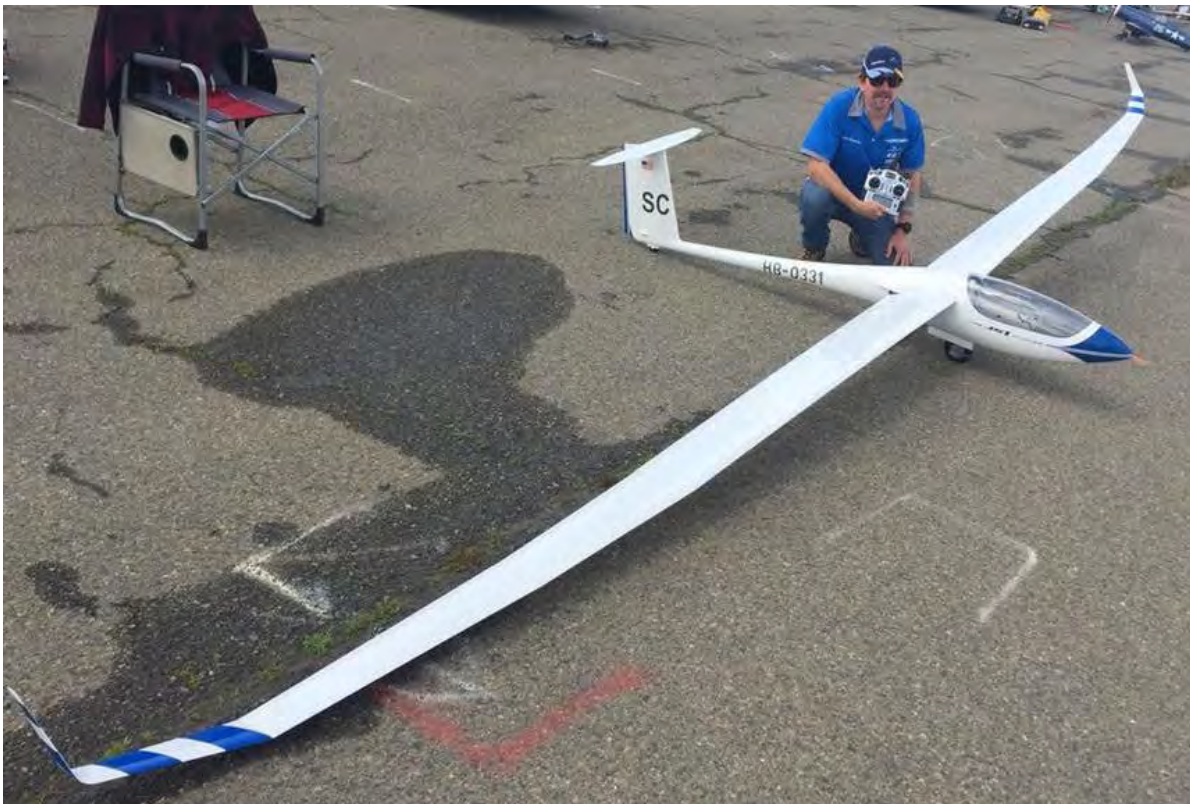
Steve Condon 1/3 scale JS1 sailplane before the maiden at Horno Field on Camp Pendleton. Brand new from LET Model. This is the second one out of the molds. Purpose built for GPS Triangle racing - it has a very thin airfoil. Flies fantastic!
