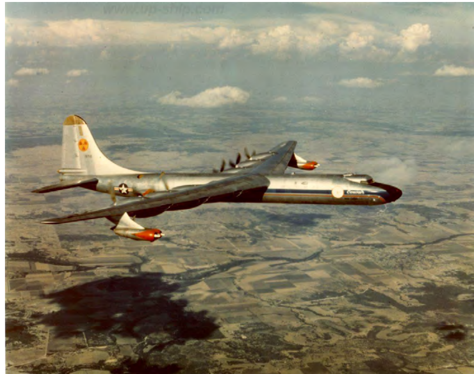
The NB-36H was a modified Convair B-36 Peacemaker that was used as a testbed for an American nuclear powered bomber.
