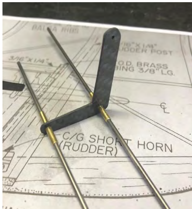
A carbon control horn made from scratch (Mark Baldacchino photo)
