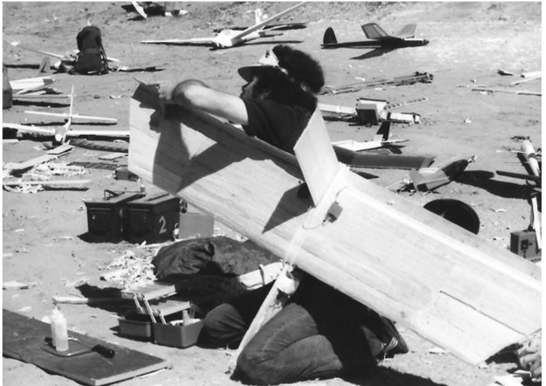
Steve Manganelli also build a flying wing for this particular contest. If you look carefully you can see how the planks of balsa were glued together to form the basis of the wing which was then sanded into the shape of an airfoil.
