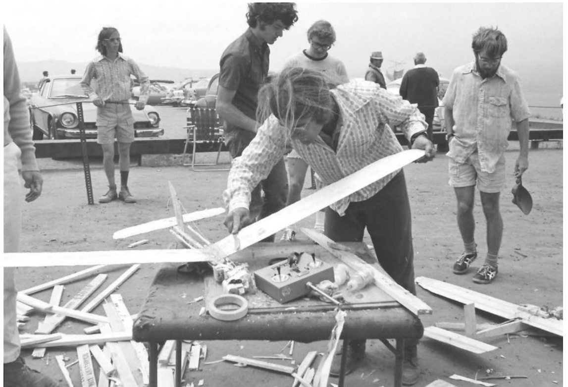
Phil Merrick uses a knife to carve an airfoil rather than sand in order to save time. Also note the wonderfully aerodynamic RC gear on the nose and the wooden pushrods.
