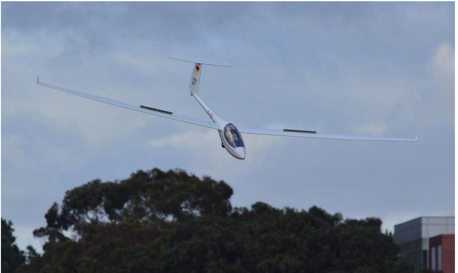
Scale ASW-27 with spoilers deployed about to land at Torrey (Greg Houck photo)
