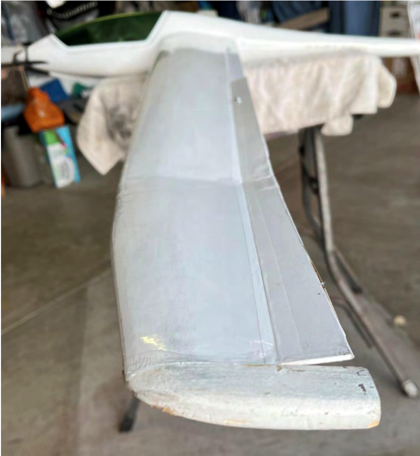
Detail of the additional wing surface serving as strip ailerons and flaps, along with the new droop tips (Marty Zimmerman photo)
