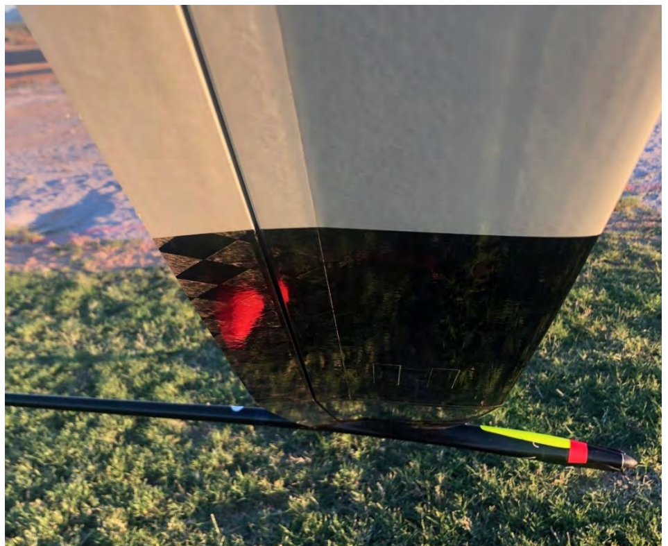
PhoenixDF float mode camber setting... +/- 15 mm measured at the root (Mike Smith photo)
