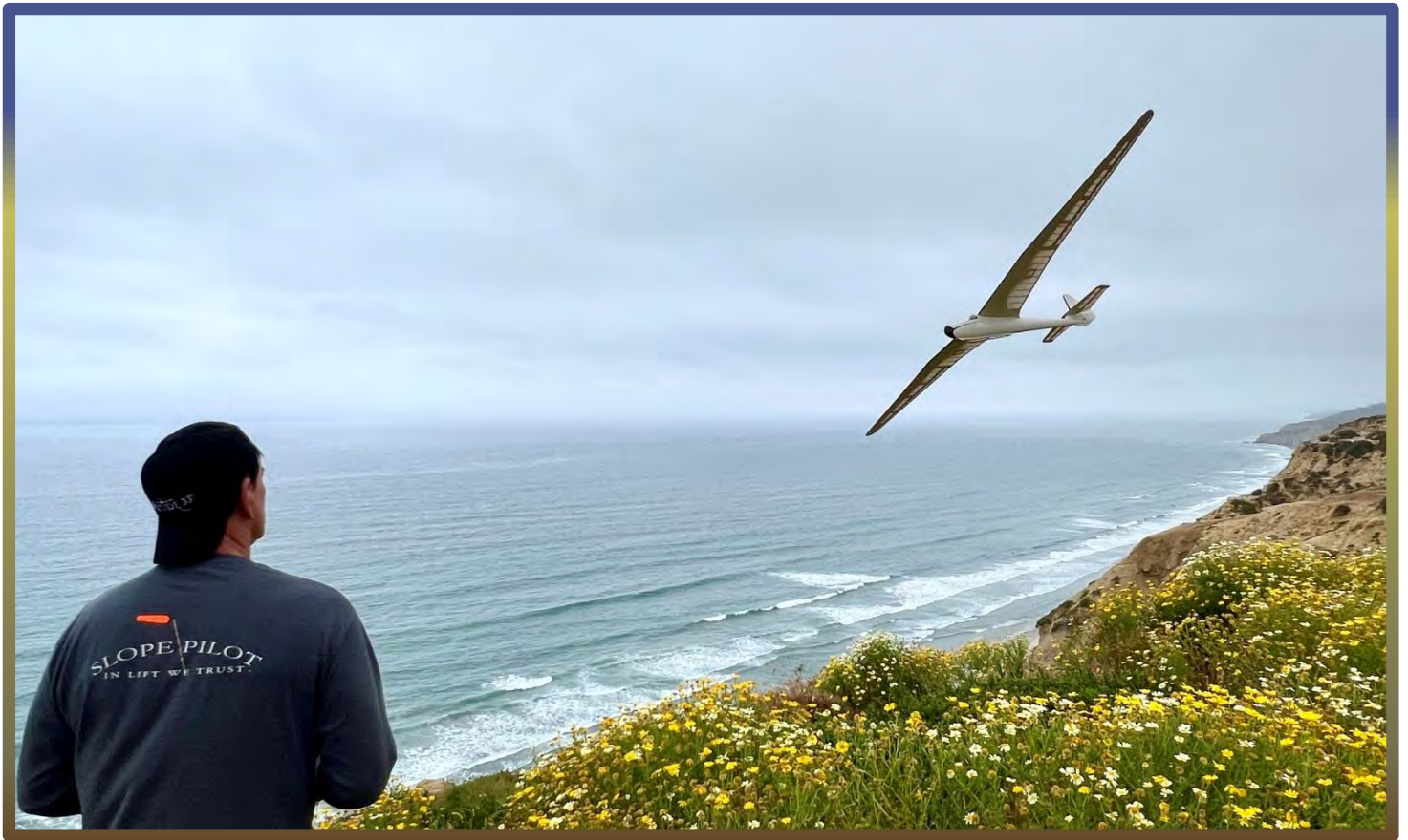
July/August Winner – Keith McLellan flying Ted Torpin's 5-meter Slingsby T13 Petrel. Built from a kit by Old Gliders; covered in dope and fabric (Bob Hirsch photo)
